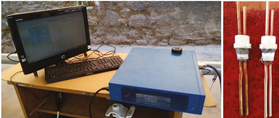
Figure 4. Equipment for stimulus-response technique.
