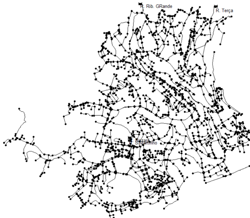
Figure 3. Calibrated hydraulic model of Funchal WSN
